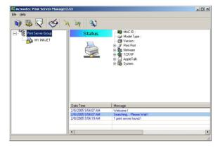
In the left pane of the window is a graphical representation of the Print Server and the printers connected to it. At the bottom of the screen is an event monitor, which lists any actions performed while using the Print Server Manager. There are a series of icons in the tool bar across the top of the window: Status, Setup, Wizard, Report, Refresh, Reboot, and Search.
